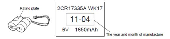
The battery can be changed with control circuit power ON. When replacing the battery with control circuit power OFF the absolute position will be erased and a machine home position return will need to be done to reestablish a home position.
