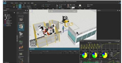
Pre-verification is performed in the digital space of a virtual factory or equipment line. This significantly reduces cost and time during the design phase.
