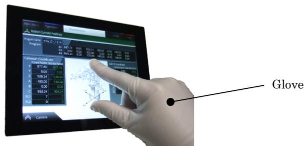
Mitsubishi Electric Color TFT-LCD module with projected capacitive touch panel
