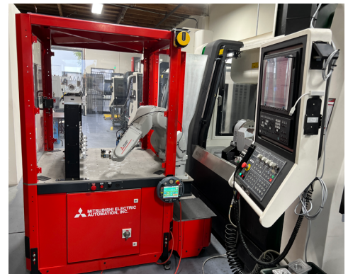
LoadMate Plus™ is an engineered robotic solution that can be used for machine tending, with an RV20, six-axis robot arm.
