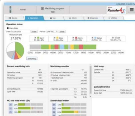
The utilization rate and operation data of each machine are displayed. Visualization and analysis helps you improve production process.
