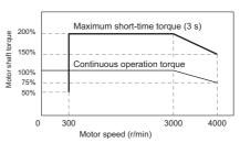
When the input voltage is low, the torque may be reduced. In the low-speed range, torque ripples or uneven rotation occur. Adjust the setting of Pr.820 Speed control P gain as required.
