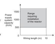
For the single-phase 200 V power input models, select the reactor whose capacity is one rank higher than the motor capacity.
