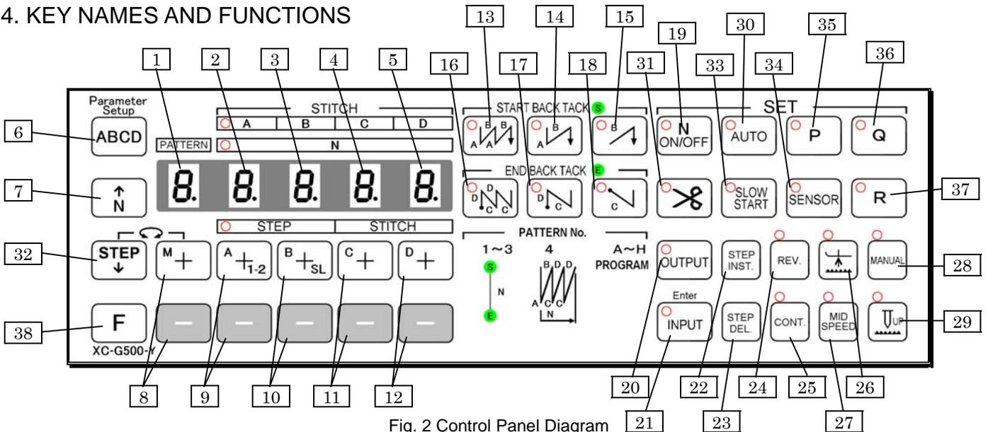
Fig. 2 Control Panel Diagram
