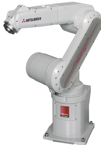
Mitsubishi Electric’s RV-12SQ robot includes a collision detection function along with communication to an iQ Platform PLC for complete system control.
