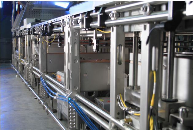
The i-Series High Performance Thermoformer from VC999 Packaging Systems is powered by Mitsubishi Electric's L Series PLC and utilizes the 1 Gbps Ethernet-based CC-Link IE Field industrial network.
