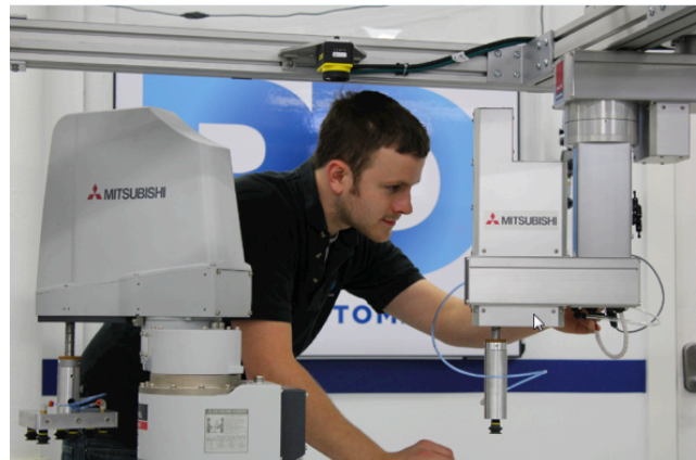
Mitsubishi Electric's SCARA robots with Cognex vision systems provide easy installation and fast programming for conveyor and vision line tracking applications.
