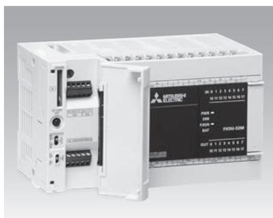
FX5U CPU module has built-in analog input/output. It contains 2-channel analog input and 1-channel analog output.
