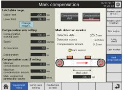
Axis setting, equipment design (cam profile, mark detection, etc.) and production management screens ensure quick and easy interaction between operators and machines.
