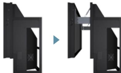
\*For ventilation requirements, leave a space of 5cm or 2 inches at the back of the display unit, against the wall.
